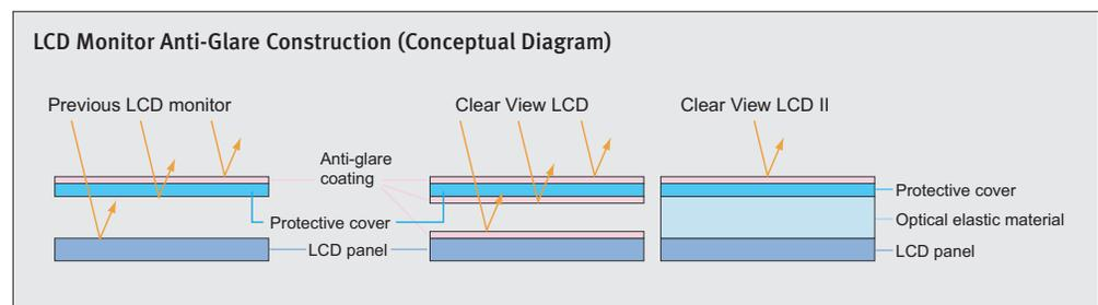
to scratching. Scratches on the protective cover that can hinder screen visibility no longer pose a problem. The EOS-1D Mark IV's LCD monitor's glass surface has an anti-reflective coating and a smudge-resistant coating. Together with the internal reflection-reduction technologies already mentioned, the LCD monitor is now easier to see even under sunny outdoor conditions.
