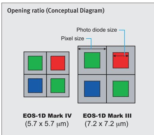
Canon's improved semiconductor fabrication technology has enabled a new method of photodiode construction. Photodiode area is optimized and photoelectric conversion efficiency is improved. This allows more light energy to be accumulated and transferred even though pixel size has been reduced.
