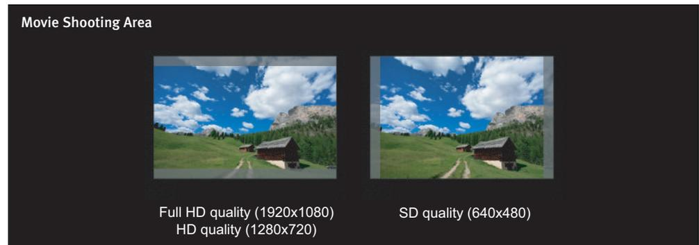
The displayed frame rate options will change automatically depending on the video output format (NTSC/PAL). Based on user requests, the frame rate has been changed to conform to the NTSC/PAL format and motion picture standard. The frame rate for HD and SD quality has been doubled compared to the EOS Rebel T1i, making videos look less jerky for fast-moving subjects and action. (The frame rate for SD quality is also twice as fast as the EOS 5D Mark II.)
