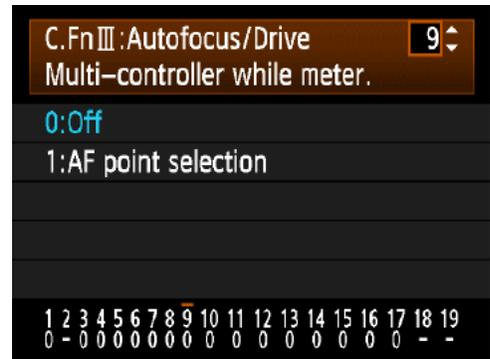
C.Fn III -9 enables AF point selection via the multicontroller while metering.
