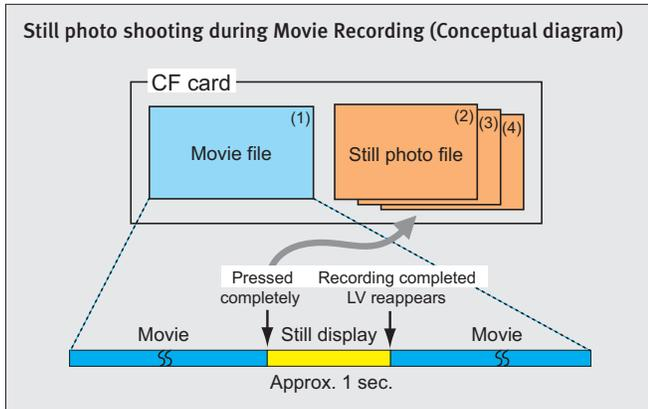
During auto exposure video shooting, exposure control for still shooting is done with a Program AE dedicated to still shooting. The ISO, shutter speed and aperture displayed on the bottom of the screen when you press the shutter button halfway are the exposure settings that will be used for still shooting. The exposure setting for video shooting is not displayed.
