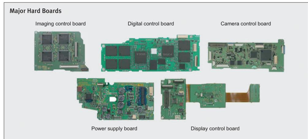
The display control board has the display IC for the display panel, viewfinder display and for the drive control of the superimposed display. It also has the motor driver IC for the shutter motor's drive control.
