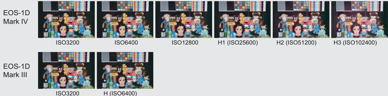
noise in the shadow areas and luminance noise are greatly reduced. The “Standard” setting obtains better noise reduction than the EOS-1D Mark III’s “Enable” setting. Thanks to improved noise reduction, a CMOS sensor with a high S/N ratio, and the DIGIC 4 Image Processor's high-speed and low-noise image development, ISO 12,800 can be included in the normal ISO range and the ISO speed can be expanded to 25,600 (H1), 51,200 (H2) and 102,400 (H3).
