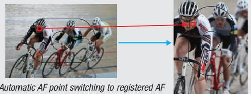
Automatic AF point switching to registered AF point when camera orientation is changed.
