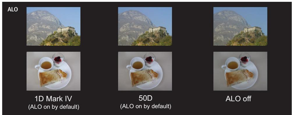
ALO works with both JPEG and RAW images. With RAW images, photographers can choose the same settings that the camera offers when processing the images in the supplied DPP software. You can select from Standard, Low, Strong or Disable. With previous EOS DIGITAL cameras having ALO, the function worked only in the P, Tv, Av and CA modes. However, with the EOS-1D Mark IV, ALO now also works in the Manual mode and bulb as well, in keeping with the idea of enhanced JPEG workflow.
