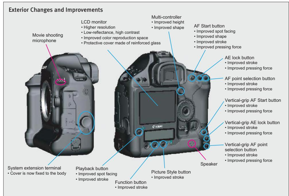
The dimensions are the same as the EOS-1D Mark III's at 156 x 156.6 x 79.9 mm/6.1 x 6.2 x 3.1 in. (W x H x D). The weight has increased by approximately 1 ounce to about 1180 g/41.6 oz. (body only) due mainly to the LCD monitor's reinforced glass.
