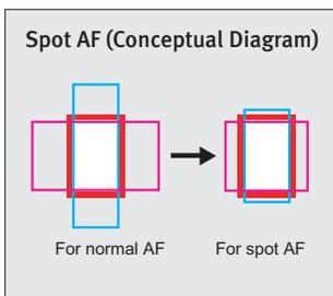
Spot AF works regardless of the AF mode and AF point selection method. It is especially effective for manual AF point selection. However, since the decrease in size may make it difficult to keep the AF point centered on an erratically moving subject, focusing might be difficult. When starting with a scene entirely out of focus, Spot AF focusing may be slow. As a reminder that Spot AF has been set, the AF point display in the viewfinder will flash brighter than normal.
