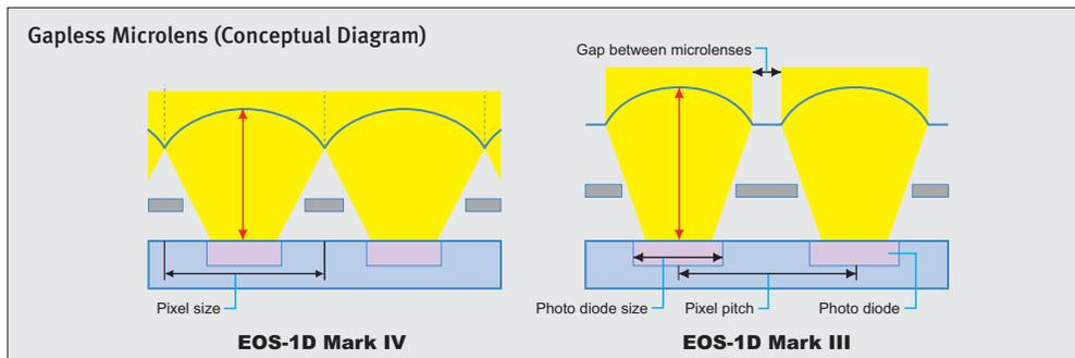
Several additional significant technical developments contribute to increased S/N performance. A new material used for the sensor unit’s RGB primary color filters improves transmittance. In addition, the circuit for applying high gain now suppresses noise from outside the sensor, improving resistance to noise and resulting in low noise even at high ISO speeds. Finally, a preamp whose internal gain has been doubled is incorporated, further increasing S/N.
