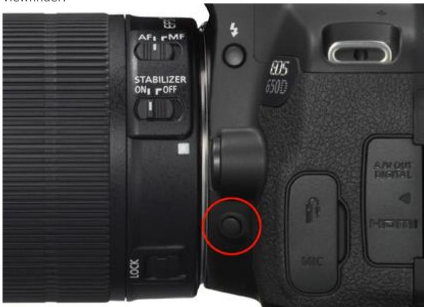
The depth-of-field button (photo above) lets you see how the image will look at the selected aperture. Wide apertures such as f/4 give a narrow depth-of-field; only a small area in front of and behind the plane of focus will appear sharp. Small apertures, such as f/16, give a wider area of apparent sharpness.
