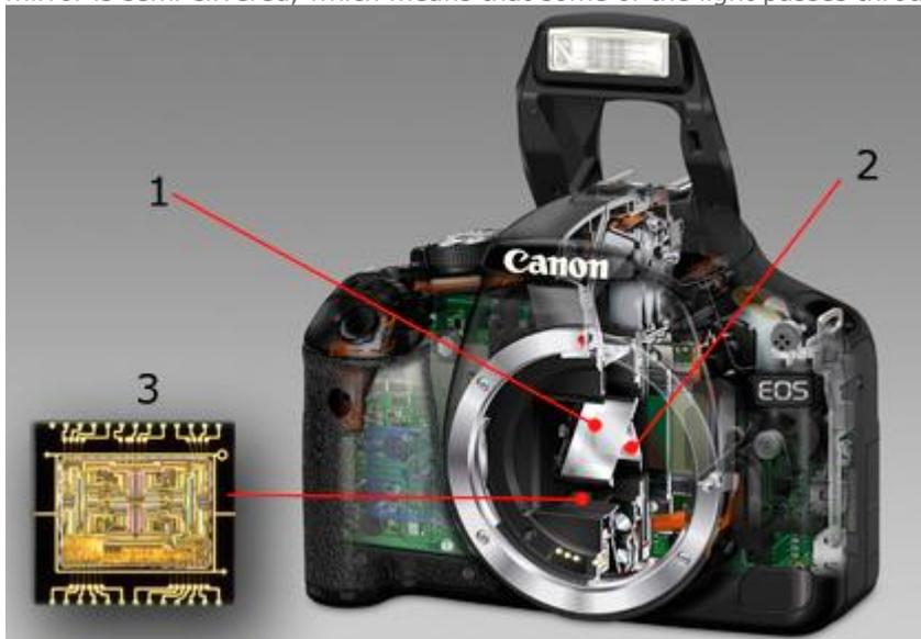
Angled behind the main mirror (1) is a smaller secondary mirror (2). This reflects light down to an AF sensor (3) in the base of the camera. This sensor looks for repeating patterns and is able to measure the amount of defocus in an image. Data is sent to the focusing motor in the lens to bring the image into focus.
